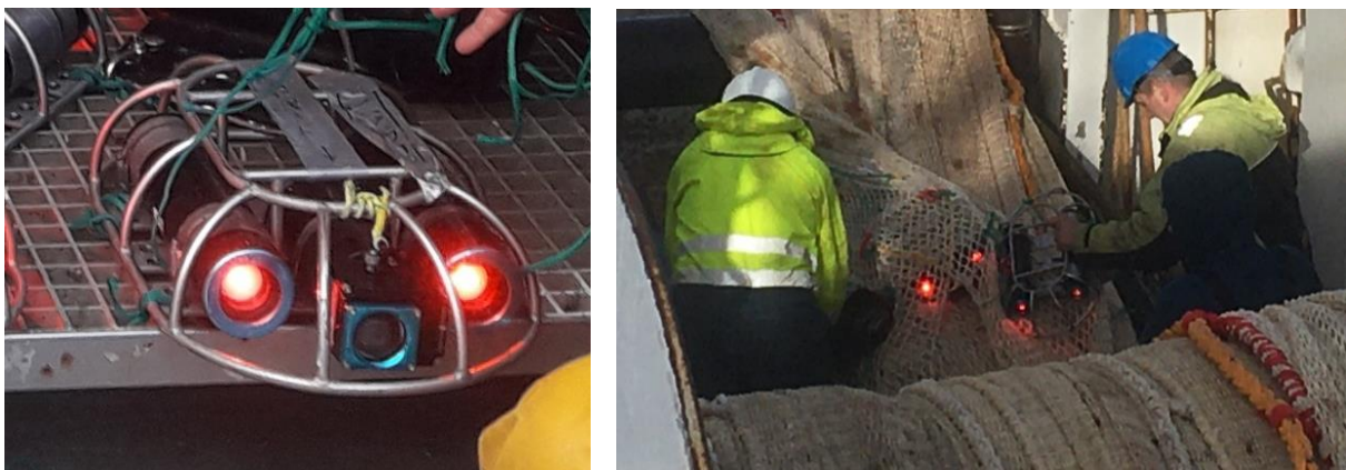
Figure A1 – “dome-frame” with camera (in a B-group housing), and with two red lights (left), and being fitted/removed from the trawl (right).
