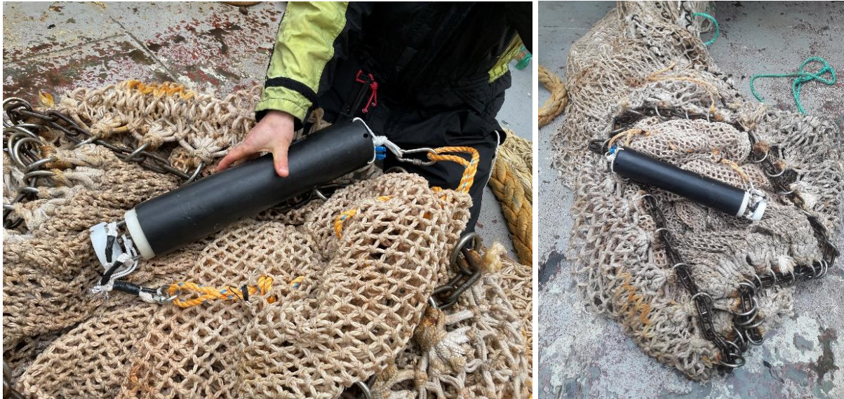
Figure 23 – Rinko oxygen logger, inside protective housing, being fitted inside the codend skirt before was coupled with the fish pump during Haul 03.
